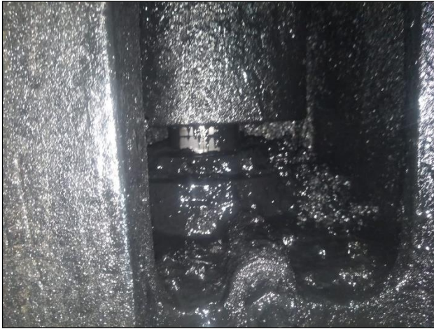
The left picture shows bad fuel quality and excessive “blowby”; the picture on the right shows “normal” running condition of the engine
