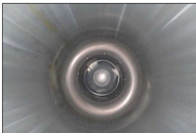
The pictures above show a cylinder liner without cold corrosion with the honing marks still visible
