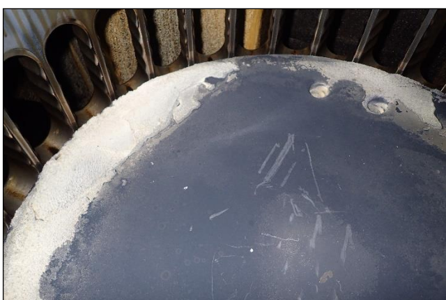
The pictures above show the effects on piston crown due to high cylinder oil feed rate; the white substances shown on the right are calcium carbonate deposits.
