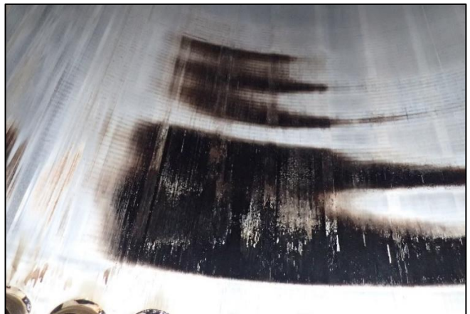
Cold Corrosion occurring on cylinder liners
