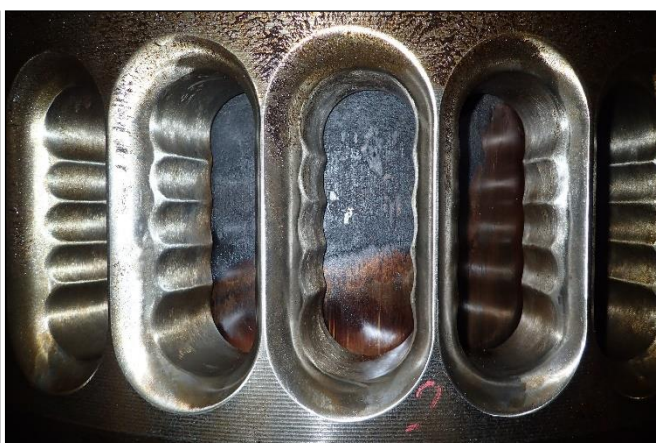
Left picture shows the piston rings with sufficient lubrication; the picture on the right shows the condition of the piston crown side with minimal carbon deposits.
