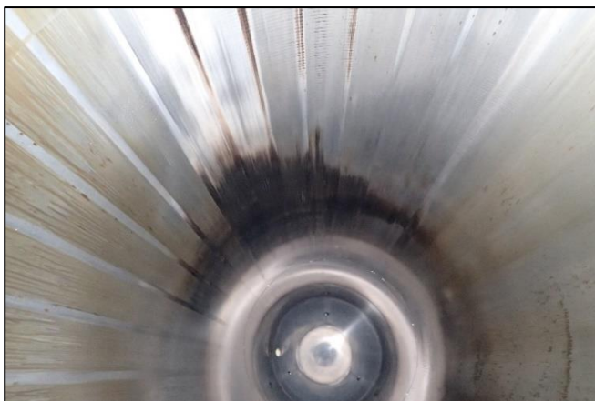
Cold Corrosion occurring on cylinder liners
