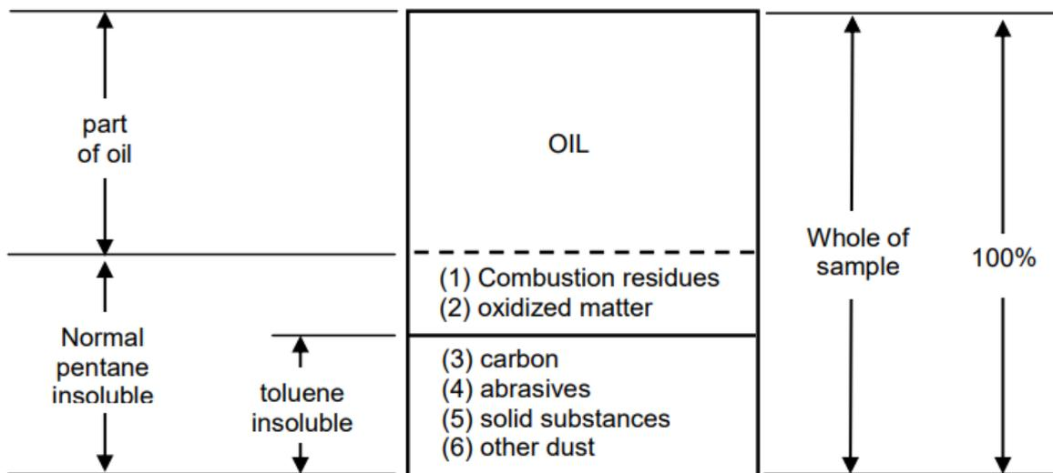
Insolubles % gives an indication of the efficiency of the purification or filtration of oil. Common test methods make use of solvents to lower viscosity and then subject the sample to centrifuge, thus, separating the total insolubles through a membrane filter.
