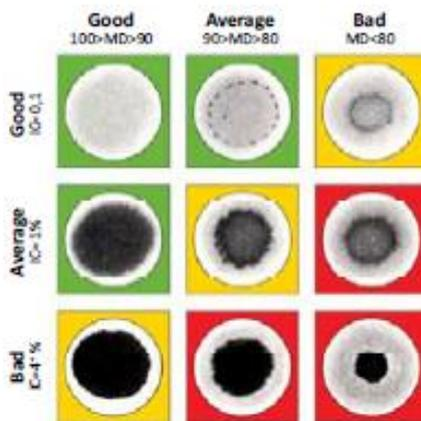
Unlike measuring soot concentration where numerous options exist, measuring dispersancy performance is a real challenge. There are two ways to approach the issue: one can attempt to measure the concentration of the dispersant additive itself, or one can measure the dispersancy performance of the oil. For routine used oil analysis, the latter offers a much more promising solution.
