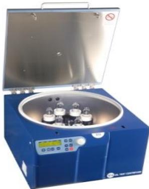
The mixture is then centrifuged to separate the insoluble material and the insoluble material is then measured to determine the percentage of insolubles. The test is then repeated using toluene instead of pentane.
