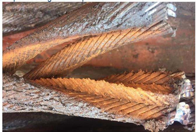
Wire ropes failure due to non-penetration of the grease to the inner core
